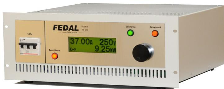
Laser power supply for solid laser is designed to work as a part of industrial, scientific or experimental units based on continuous wave solid lasers or pulse lasers operating in the Q-switched mode (with acoustooptic shutter). The power supply can be used in a wide range of applications, including laser metal cutting, engraving, scribing of ceramic and semiconductor wafers, resistor trimming and laser beam marking..
